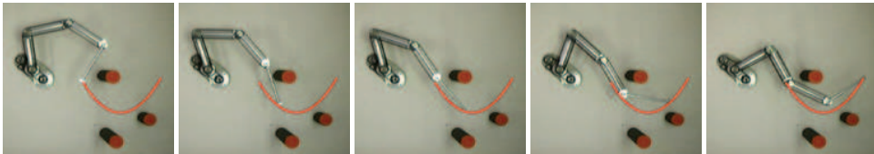
Fig. 15. Planar 4DOF manipulator tracking a path in an unstructured environment with three obstacles using velocity-based control (sampled every 1s)
