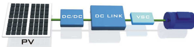
Fig. 13. Voltage Source Converter Interface
