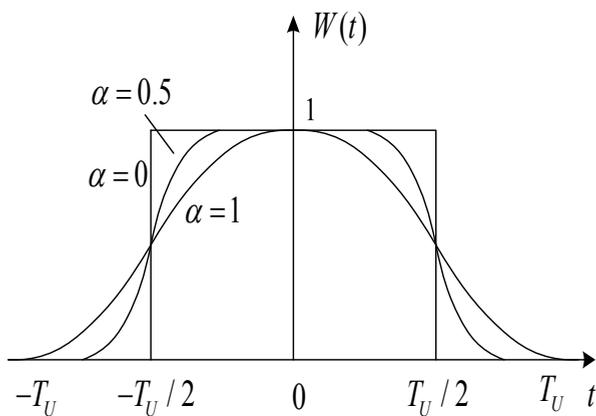
Fig. 14. Raised cosine window function  $w(t)$  depending on roll-off factor  $\alpha$
