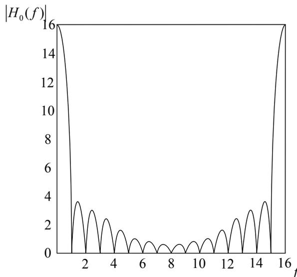
Fig. 10. Frequency response of a DFT filter ( $n = 16$ )
