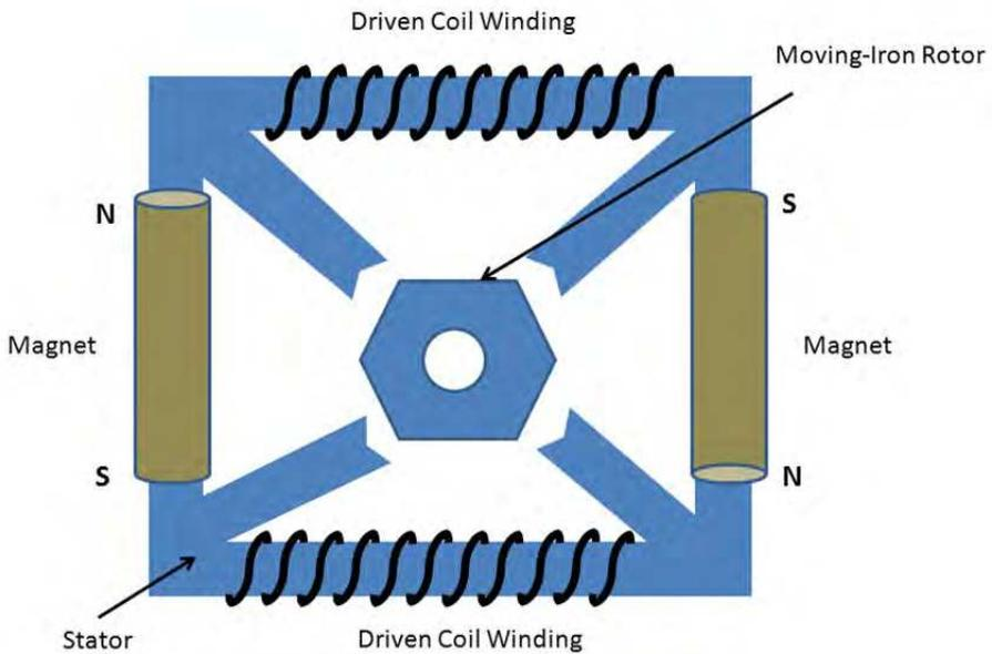
Fig. 2. Moving-Iron Galvanometer
