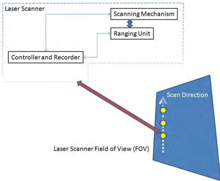
Fig. 1. Terrestrial Laser Scanning System Components
