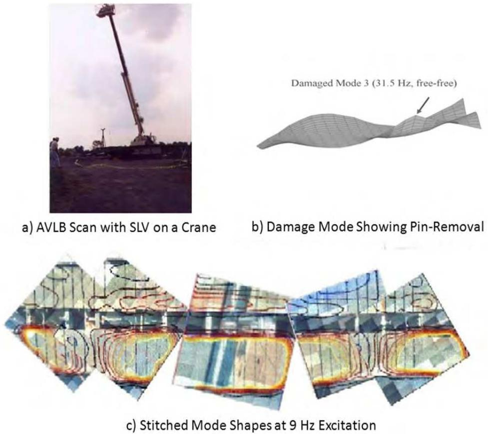
Fig. 11. SLV Scan of AVL Bridge
