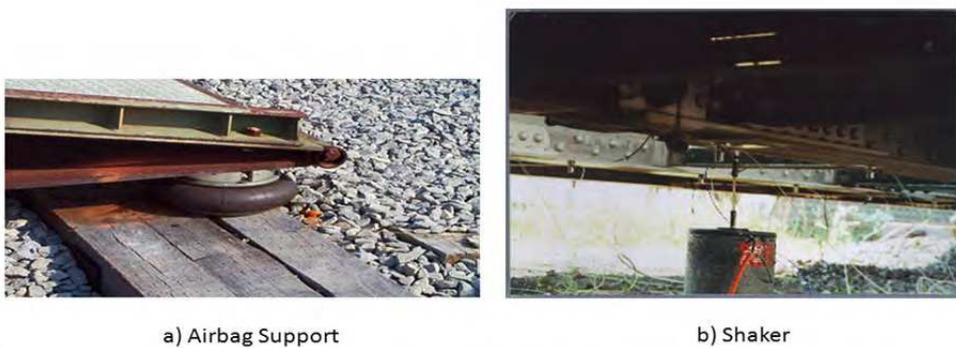
Fig. 12. Testing Setup: a) Airbag and b) Shaker
