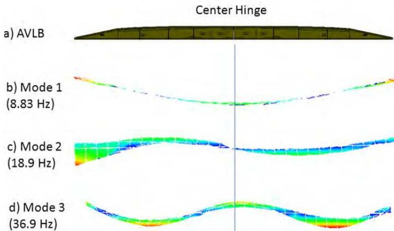
Fig. 13. Modal Behaviors of AVL B: a) AVL B; b) Mode 1; c) Mode 2; d) Mode 3
