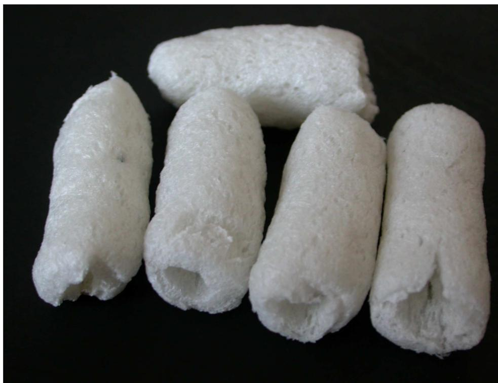
Fig. 1. Extruded starch foams.
