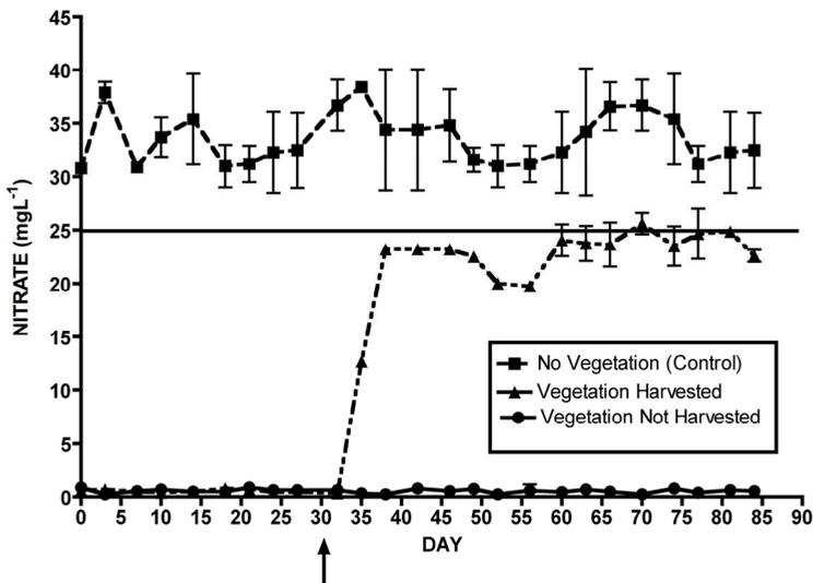
Mean  $\pm$  S.D. of effluent nitrate concentration in RVFB treating synthetic tile water ( $25 \text{ mgL}^{-1} \text{ NO}_3\text{-N}$  initial concentration: solid line). Plants were harvested in the 30<sup>th</sup> day of the experiment (arrow).
