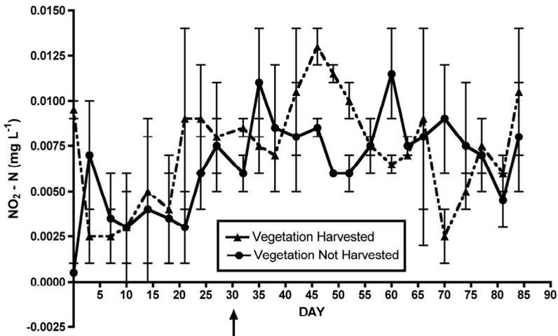
Mean  $\pm$  S.D. of effluent nitrite-N concentration in RVFB treating synthetic tile water. Plants were harvested in the 30<sup>th</sup> day of the experiment (arrow).
