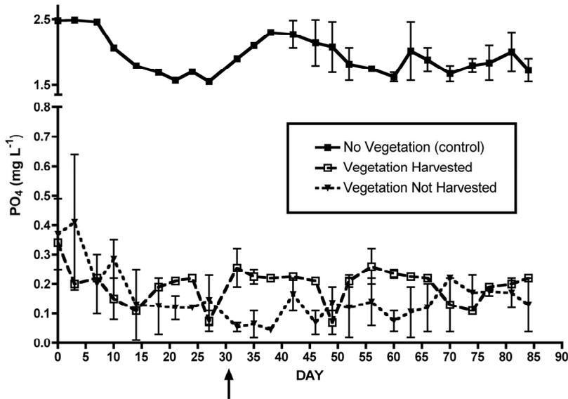
Mean  $\pm$  S.D. of effluent phosphate ( $\text{PO}_4$ ) concentration in RVFB treating synthetic tile water. Plants were harvested in the 30<sup>th</sup> day of the experiment (arrow).
