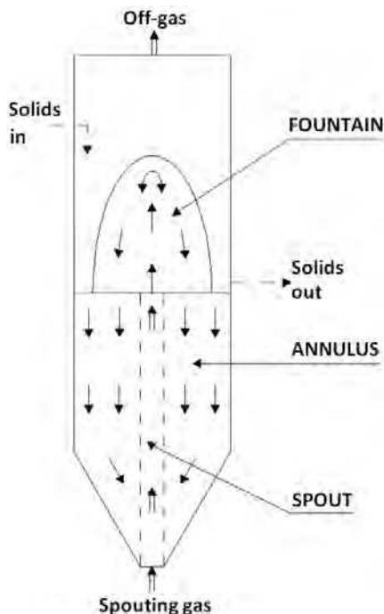
Fig. 3. Schematic of a spouted bed
