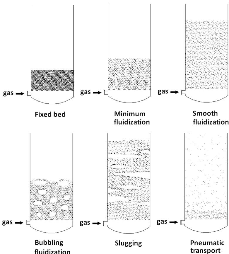
Fig. 1. Schematic representation of various fluidization regimes
