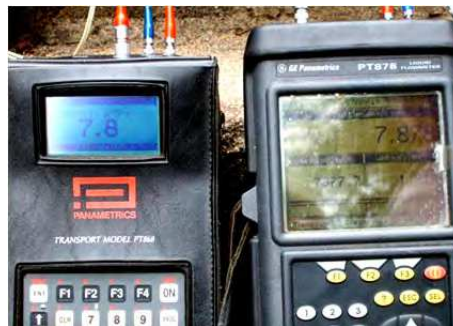
Fig. 10. Electronic devices to perform Ultrasonic measurements.
