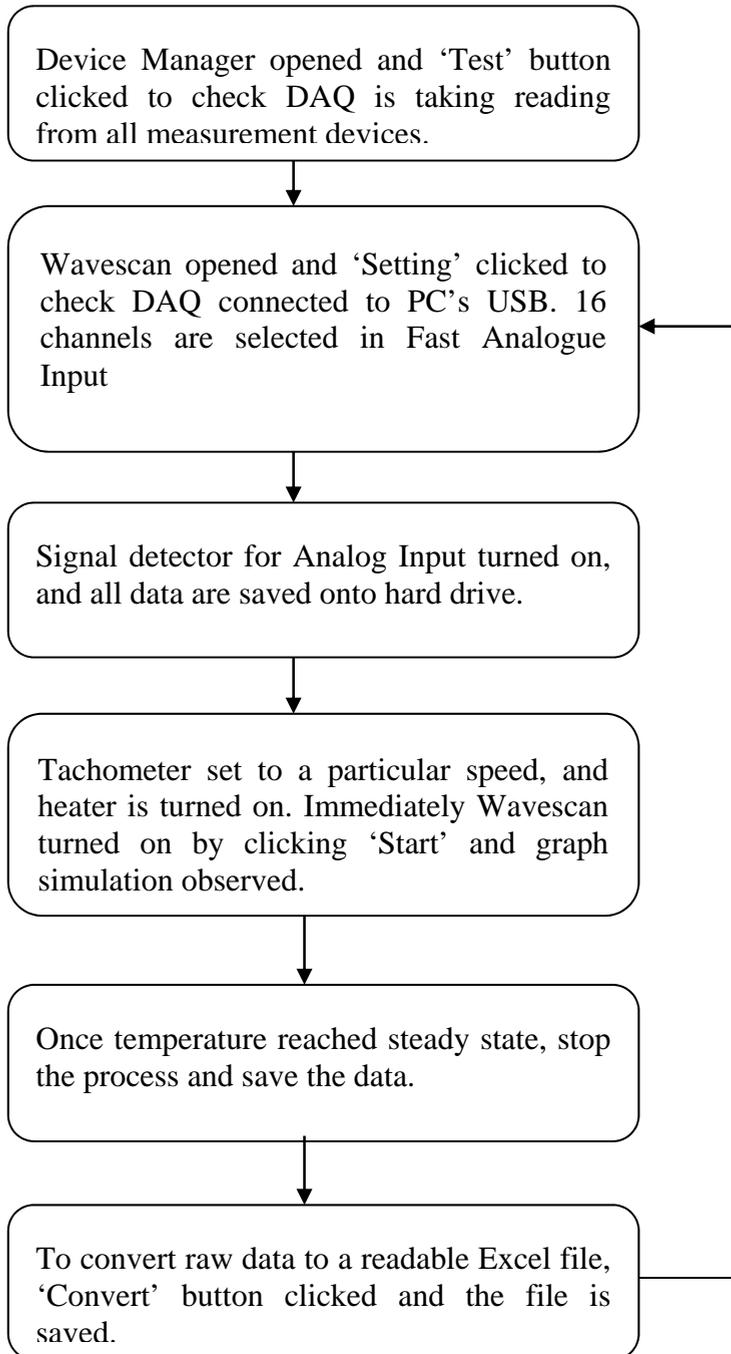
Fig. 11. Flow chart of software evaluation procedures
