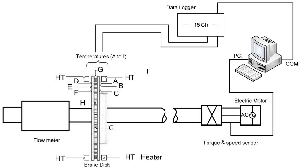
Fig. 2. Ventilating brake disk experimental rig
