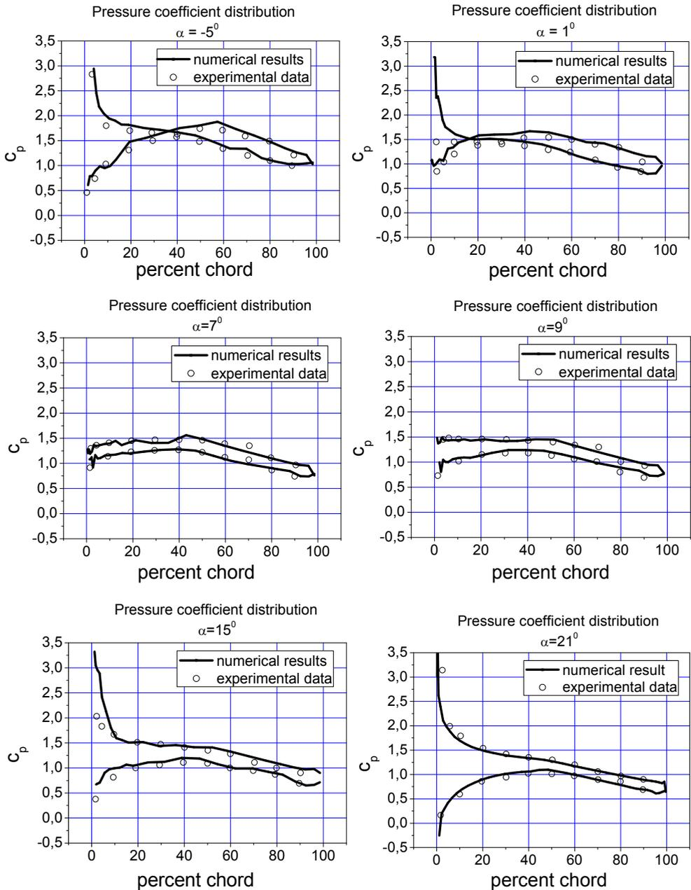
Fig. 10. Pressure coefficient distribution over the NACA 65-410 compressor cascade profile at different  $\alpha$  (angle of attack) ( $\beta_f=30^\circ$ ,  $Re=2.45E5$ , and  $v_{inf, inlet}=29$  m/s). The experimental data are from (Emery et al., 1958)
