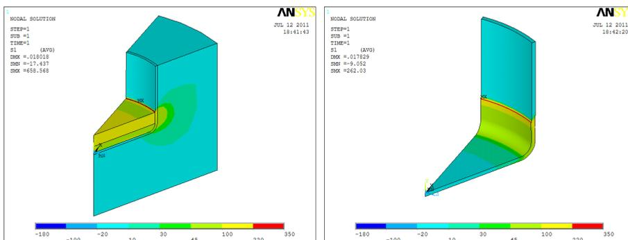
Fig. 6. First principal stresses ( $\sigma_1$ - MPa) for first layer in three-layers horizontal incremental technique - restoration on the left and interface on the right
