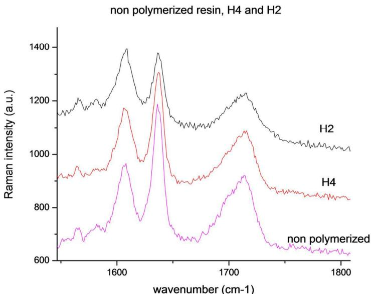
Fig. 4. Raman test results for XL3000 polymerization device and thicknesses of 2 mm (H2-G1) and 4mm (H4-G3)
