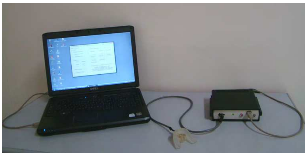
Fig. 3. Portable device for measuring the force of the tongue: Portable FORLING.
