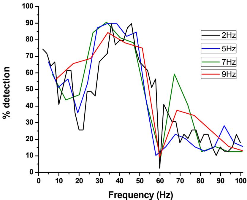
Fig. 7. Percentage of volunteers for whom the stimulation response was detected using the MSC ( $M = 200$  epochs) for the frequencies from 2 to 100 Hz at the derivation [Cz] for the stimulation frequencies 2, 5, 7, 9 Hz.
