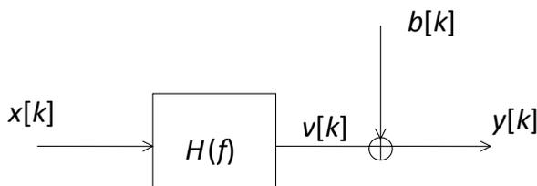
Fig. 1. Linear Model of evoked potential generation:  $x[k]$  is the stimulus,  $H(f)$  is the frequency-domain transfer function of the sensory pathways,  $v[k]$  is the stimuli-response,  $b[k]$  is the background EEG and  $y[k]$  is the measured EEG.
