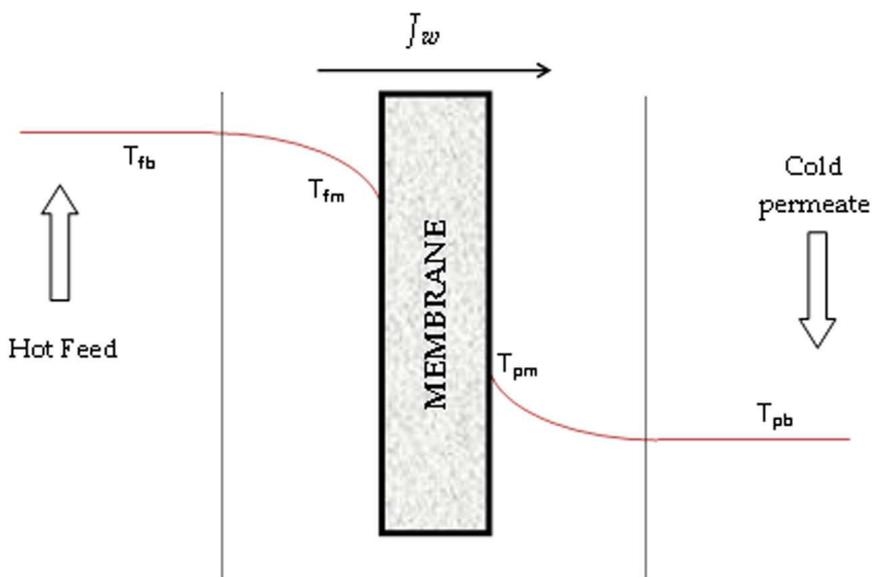
Fig. 3. Schematic diagram of temperature polarization in MD.  $T_{fm}$ ,  $T_{pm}$ ,  $T_{fb}$  and  $T_{pb}$  are membrane surface temperatures and fluid bulk temperatures at the feed and permeate sides, respectively.
