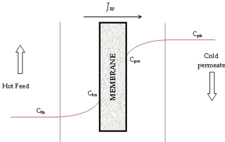
Fig. 4. Schematic diagram of concentration polarization in MD.  $C_{fm}$ ,  $C_{pm}$ ,  $C_{fb}$  and  $C_{pb}$  are membrane surface and bulk solute concentrations at the feed and permeate sides, respectively.
