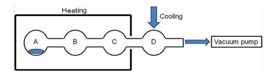
Fig. 2. Sketch of bulb-to-bulb distillation apparatus.
