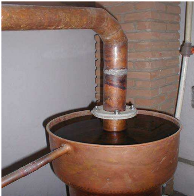
Fig. 12. Details of a cooling system on top of a hood-like column (CRD B, Paraty-RJ).
