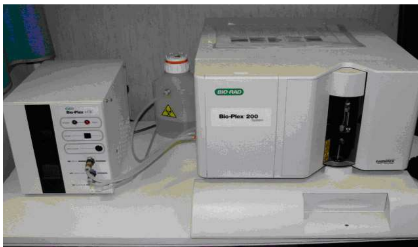
Fig. 3. Suspension array system with high throughput put fluidics system.
