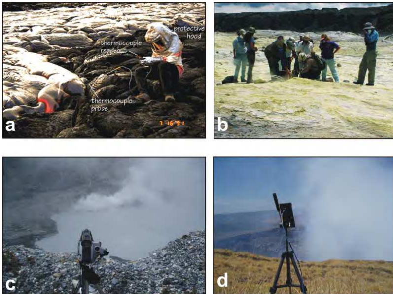
Fig. 1. Different modes for temperature and volcanic gas sampling. Conventional in situ measurements of (a) the temperature of Hawaiian pāhoehoe lava flow fields (photo by P. Mougini-Mark, volcano.oregonstate.edu), and (b) volcanic gas from the summit fumarole field of Kīlauea volcano in 2005. In (c) and (d) ground-based thermal imagery of the Laguna Caliente crater lake (Poás volcano, Costa Rica; 2009) and UV-DOAS measurements of the Santiago crater (Masaya volcano, Nicaragua; 2009) volcanic plume, respectively.
