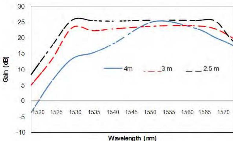
Fig. 21. Gain spectrum of the C-band EDFA
