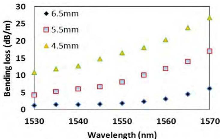
Fig. 13. Bending loss spectral for different bending radius
