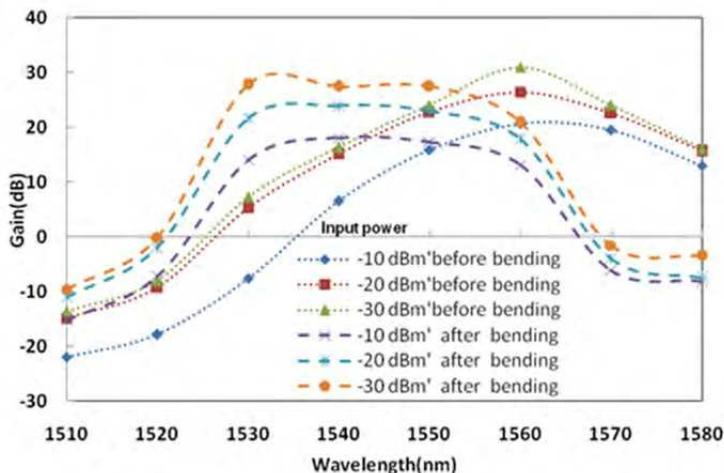
Fig. 9. EDFA gain spectra; with and without acro bending at various input signal power.
