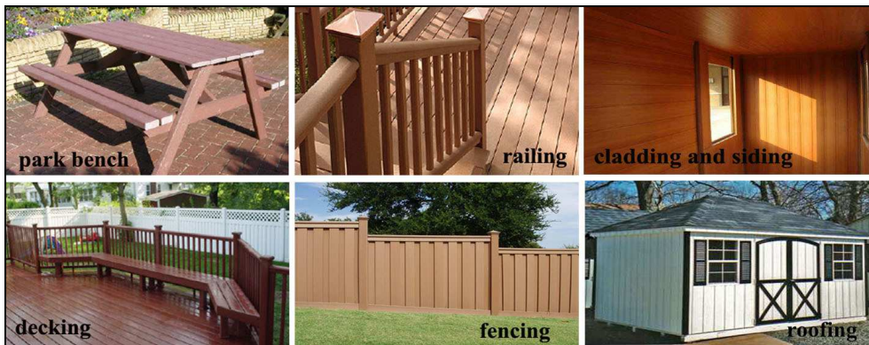
Fig. 2. Applications of natural fiber reinforced plastics in building products.
