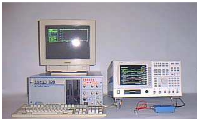
Fig. 1. Component of AE system (Prateepasen A., 2007)
