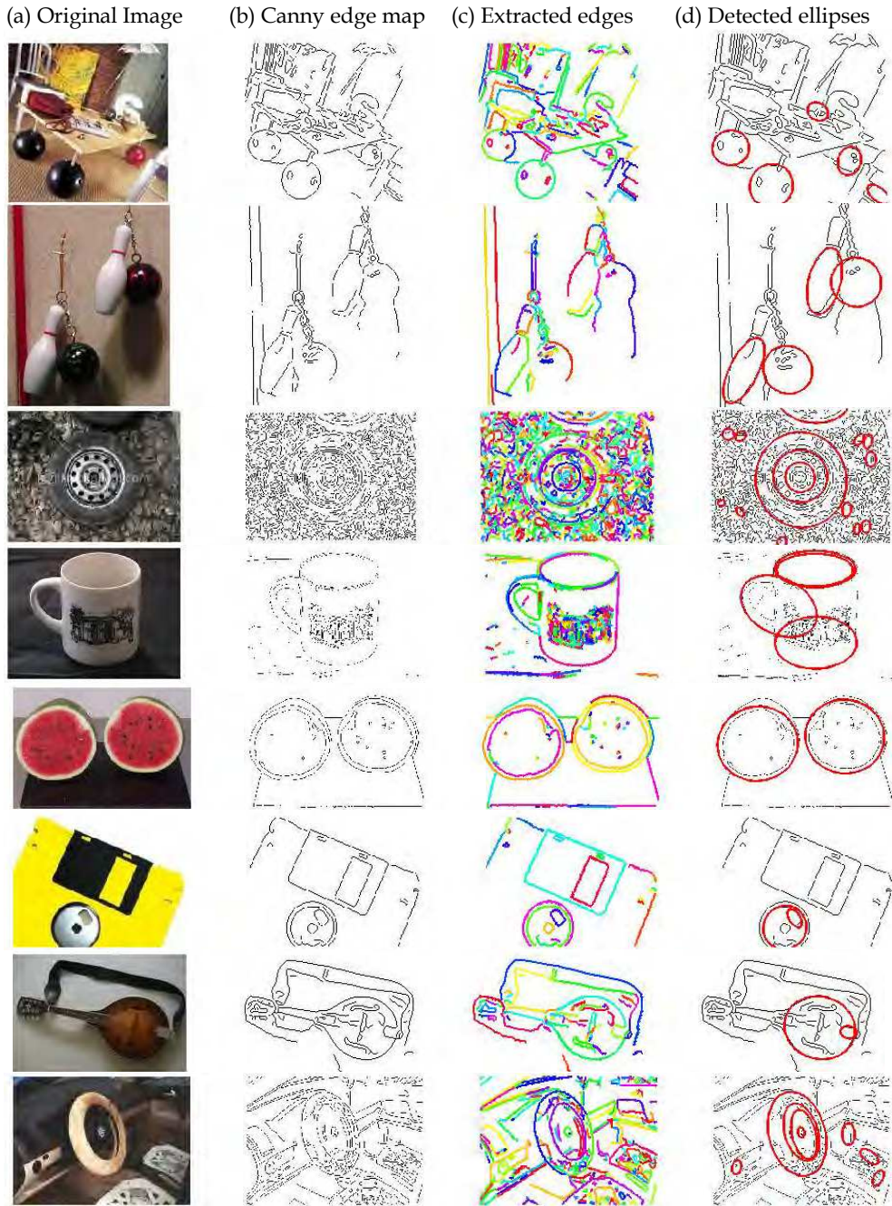
Fig. 13. Examples of real images and ellipse detection using the proposed method (continued).
