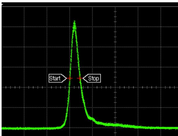
Fig. 10. Experimental photodiode impulse response (horizontal scale 25 ps/div.)
