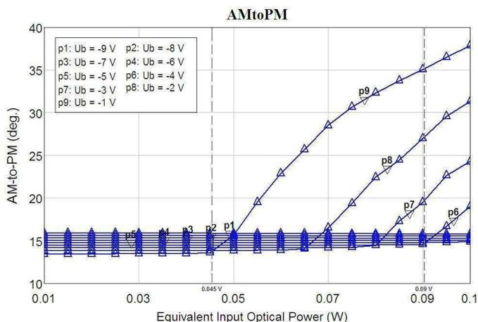
Fig. 12. Photodiode power to phase conversion characteristics
