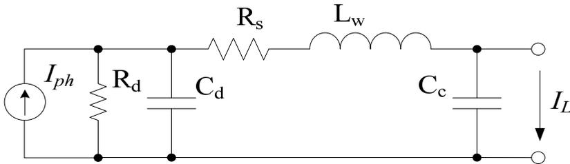
Fig. 8. The p-i-n photodiode electrical equivalent circuit
