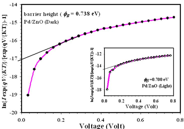
Fig. 14.  $\ln\{I \exp(qV / \{kT\}) / [\exp(qV / \{kT\}) - 1]\}$  vs V (under dark condition) of the fabricated ZnO MSM PD with Pd electrodes on PPC substrate. The inset shows  $\phi_B$  calculation under illumination
