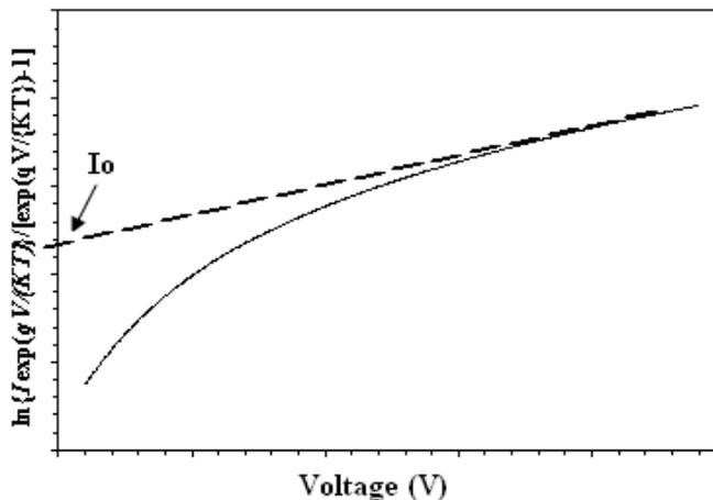
Fig. 3.  $\ln\left\{I \exp(qV / \{KT\}) / [\exp(qV / \{KT\}) - 1]\right\}$  vs.  $V$  of a MSM PD
