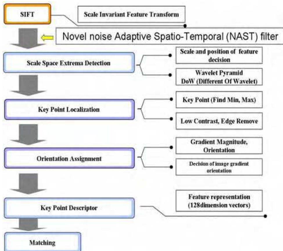
Figure 1. Conceptual flowchart of the whole structure
