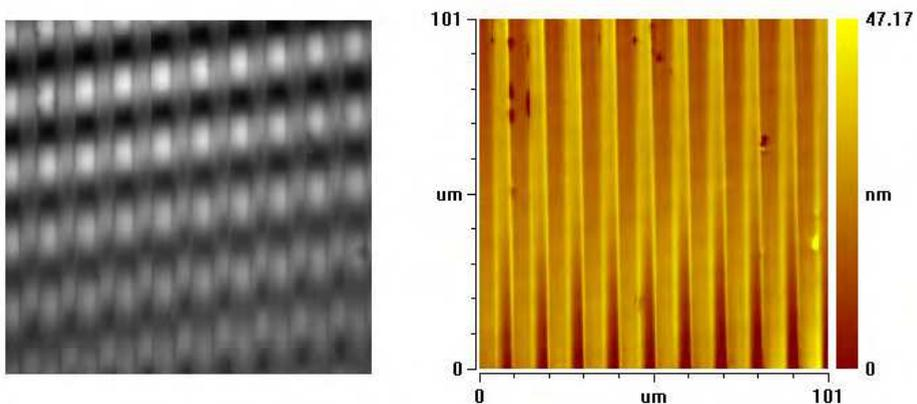
Fig. 6. Optical profilometer fringe pattern and topography images of the sample of figure 5. It is clear that the height dimensions are wrong because of the confusion of fringe order.
