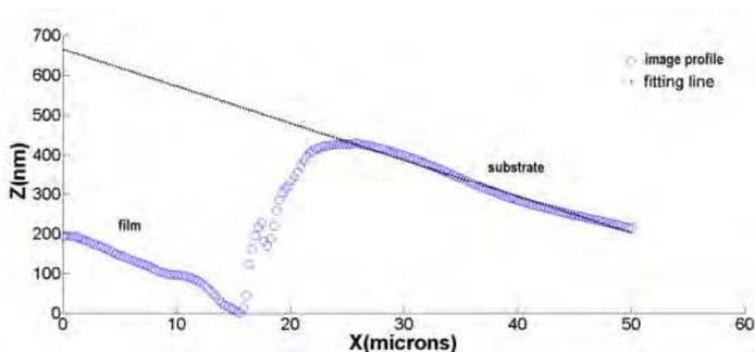
Fig. 9. Schematic representative of image fitting for tilt removal.
