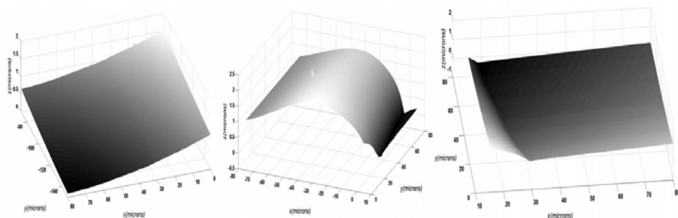
Fig. 12. Successive atomic force microscopy images of the boundaries of the photoresist film at the same region as in figure 11.
