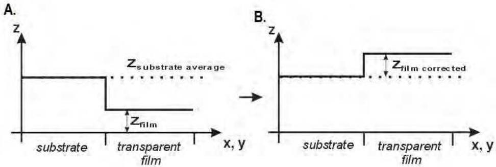
Fig. 3. 2D schematic presentation of (A) the initial image and of (B) the corrected image.
