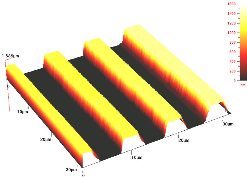
Fig. 5. 3D topography image of the sample with graded strips taken by atomic force microscopy. The steps are formed by sharp edges of 1.2 μm height
