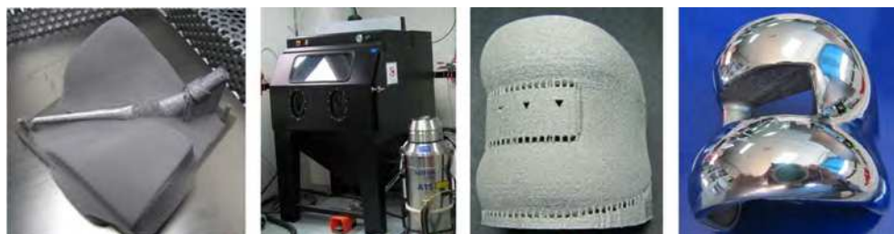
Fig. 13. Implant post-processing. From left to right: hip stem still involved by the powder bed; powder recovery system; knee implant as taken out from the machine and after support removal and hand polishing.
