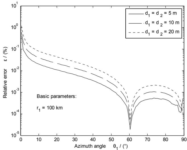
Fig. 5-2. Relative calculation error: different baseline lengths.
