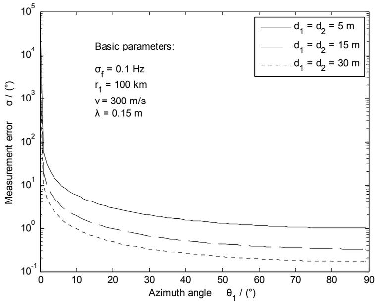
Fig. 5-4. Measurement errors: different baseline lengths.
