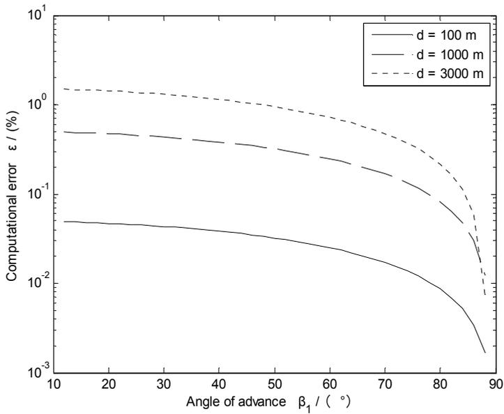
Fig. 3-2 Relative calculation error curve against advancing angle for radial distance with different displacement.
