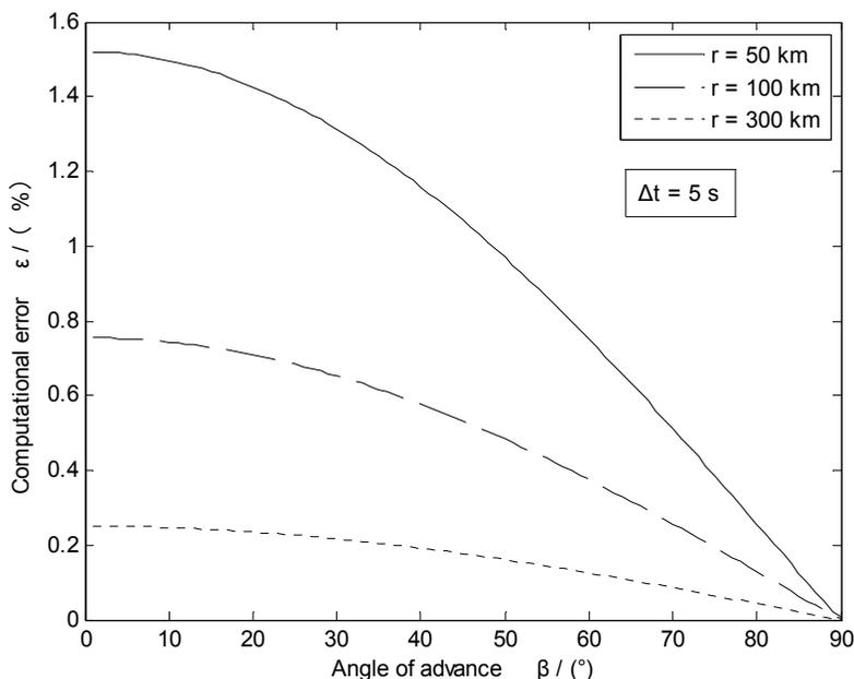
Fig. 2-8. Relative calculation error curve of Doppler changing rate against advancing angle in different radial distance
