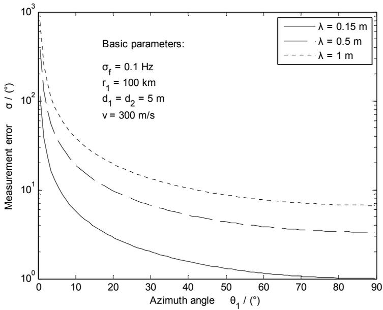
Fig. 5-6. Measurement errors: different wavelengths.
