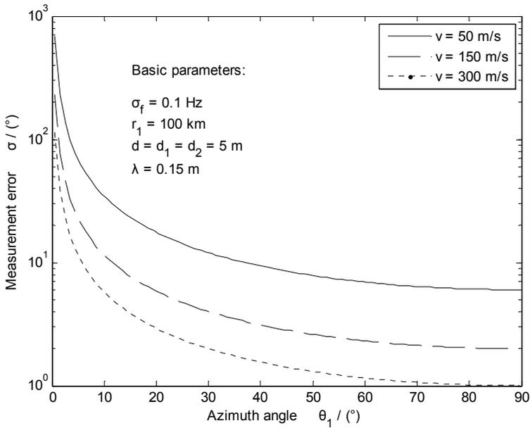
Fig. 5-7. Measurement errors: different flight speeds.
