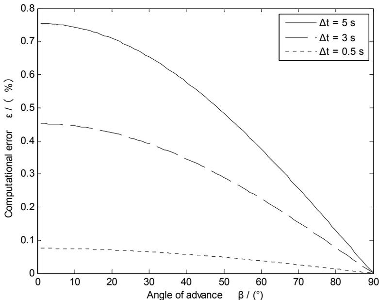
Fig. 2-7. Error curve of Doppler rate against advancing angle in different detecting times.
