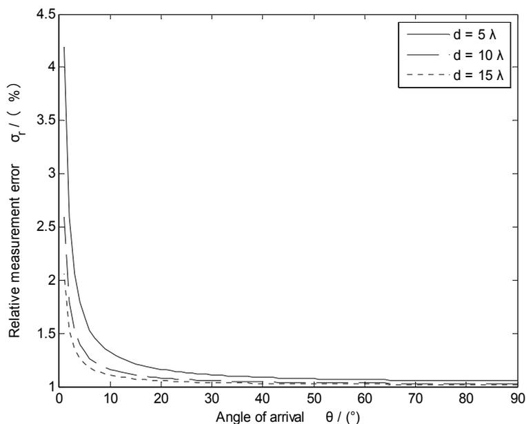
Fig. 2-6. Relative measurement error of Doppler shift.
