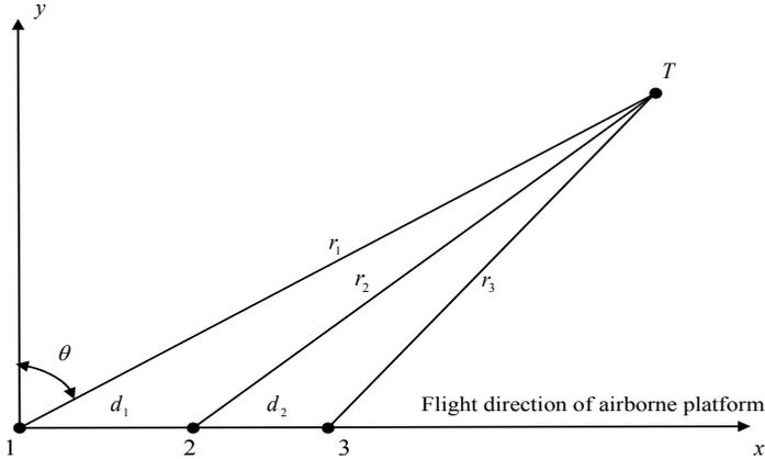
Fig. 2-2. One-dimensional array with double baseline.
