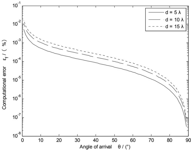
Fig. 2-3. Computational error of Doppler shift with different baseline lengths.
