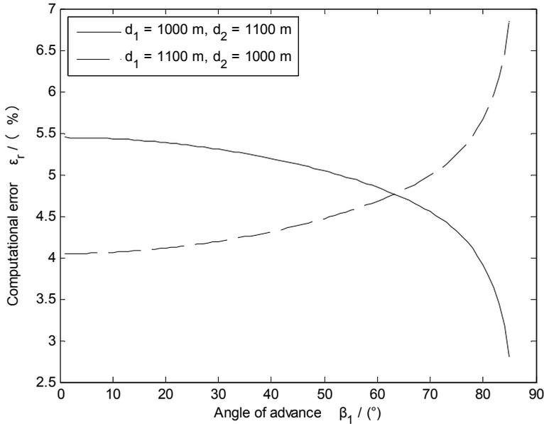
Fig. 3-8. Computational error of ranging formula in unequal spaced detection.
