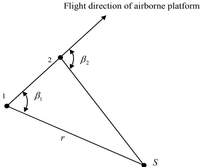
Fig. 3-1. Geometric relationship used for mobile ranging system.
