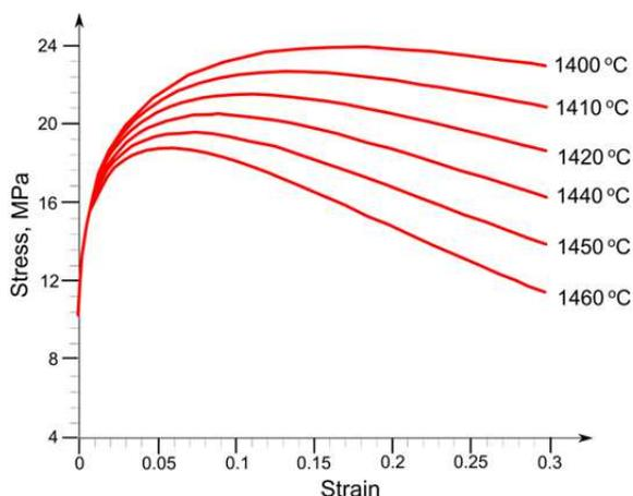
Fig. 5. Stress-strain curves at several temperature levels from the range of 1400-1450°C (S355J2G3So grade steel, quasi-static process – strain rate 1 s<sup>-1</sup> (Glowacki & Hojny, 2010).
