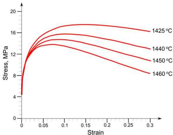
Fig. 4. Flow stress vs. strain at several temperature levels for 18G2A steel grade deformed during quasi-static process – strain rate 1 s<sup>-1</sup> (Glowacki & Hojny, 2010).
