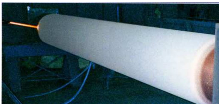
Fig. 8. Paper machine roll coated by NiCrBSi (self fluxing alloy) Vuoristo and Nysten, (2007) .
