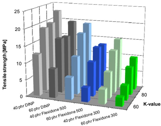
Fig. 6. Tensile strength of flexible PVC sheets with various concentrations of Flexidone 300, Flexidone 500 and DINP in PVC grades with different K-values.
