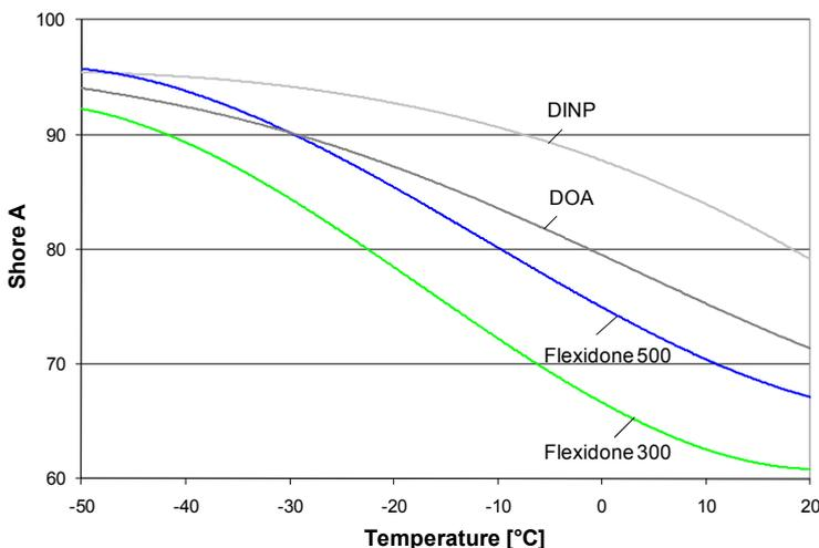
Fig. 5. Variation of Shore A values at temperatures between +20°C and -50°C for samples with 60 parts of Flexidone 300, 500, DOA (dioctyl adipate) and DINP.
