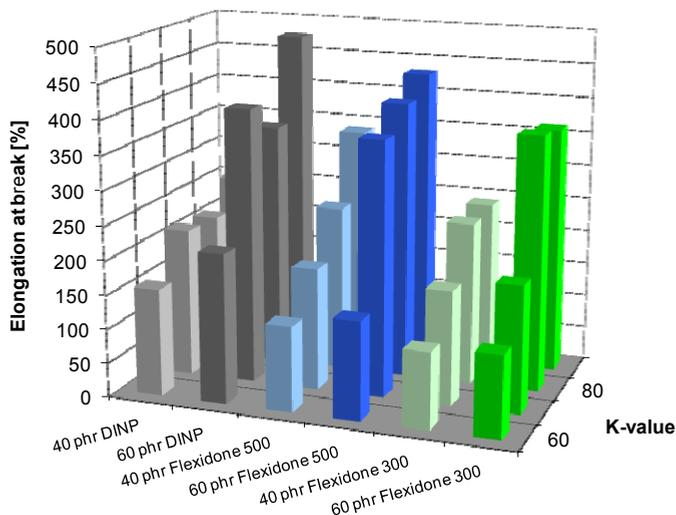
Fig. 7. Elongation at break for soft PVC sheets with various concentrations of Flexidone 300, Flexidone 500 and DINP in PVC of different K-values.
