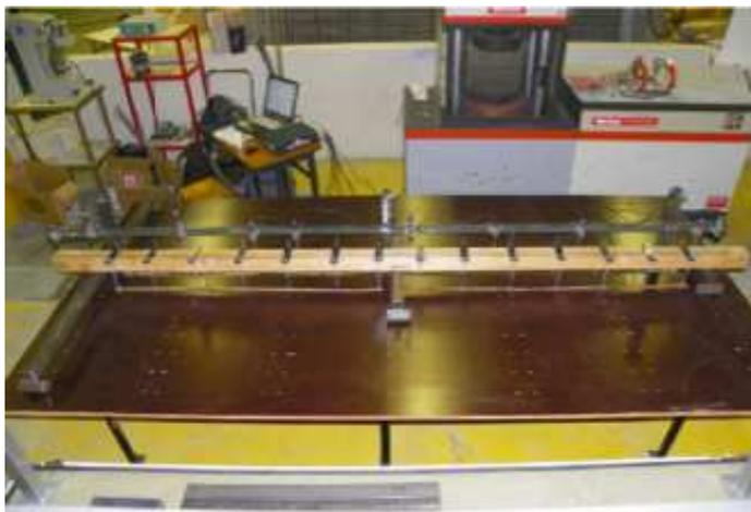
Fig. 5. Experimental device reproducing the soil-structure interaction for a two-span continuous beam.
