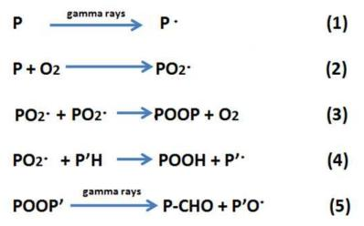
Fig. 10. Polyolefins oxidation caused by gamma sterilization
