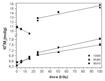
Fig. 14. Reciprocal of M<sub>v</sub> as a function of the irradiation dose of PVC and PVC/PS blends
