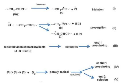
Fig. 7. Effects of gamma irradiation on PVC molecule
