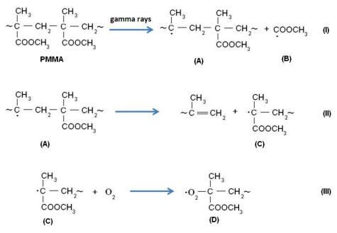
Fig. 8. Radiolytic degradation of PMMA
