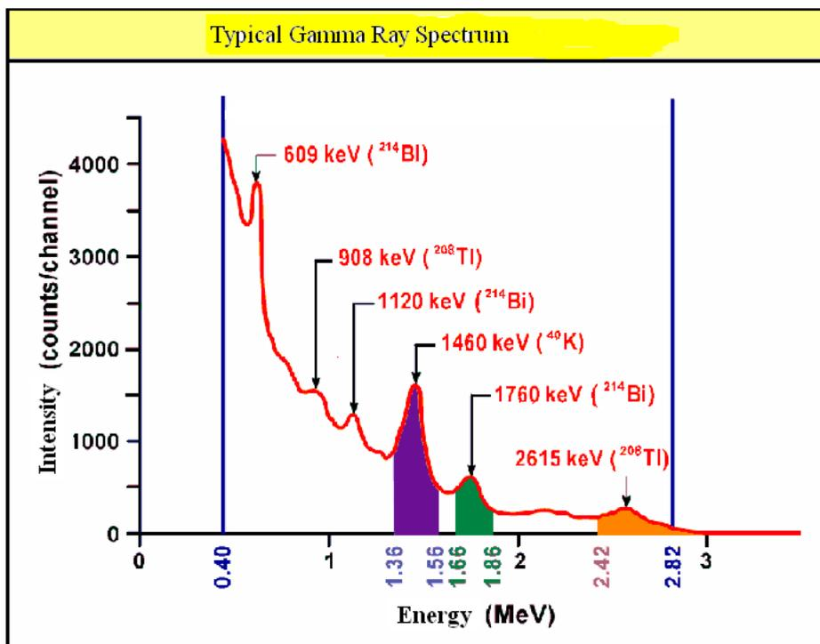
Fig. 3. Typical Gamma Ray Spectrum
