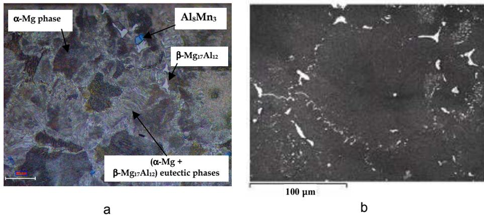
Fig. 3. a) Microstructure of the base metal, solid solution  $\alpha$ -Mg and ( $\alpha$ -Mg +  $\beta$ -Mg<sub>17</sub>Al<sub>12</sub>) eutectic phase and precipitates (OM), b) Microstructure of the Heat Affected Zone (HAZ) by SEM (Kouadri & Barrallier, 2006, 2011)
