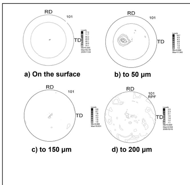
Fig. 7. Evolution of the crystallographic texture (pole figure 101) from the surface to a depth of 200  $\mu\text{m}$ : a) Texture to the surface, b) Texture to 50  $\mu\text{m}$ , c) Texture to 150  $\mu\text{m}$ , d) Texture to 200  $\mu\text{m}$  (Kouadri & Barrallier, 2006, 2011).
