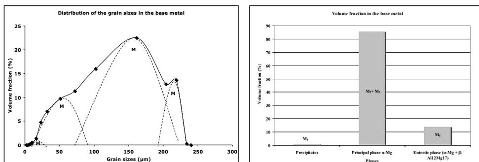
Fig. 5. (a) Statistical distribution of the grain sizes of AZ91 alloys in the base metal. (b) Volume fraction of the  $\alpha$ -Mg grains, of the eutectic ( $\alpha$ -Mg grains  $\beta$ -Mg<sub>17</sub>Al<sub>12</sub>) phase and of the precipitates in the base metal (Kouadri & Barrallier, 2011).
