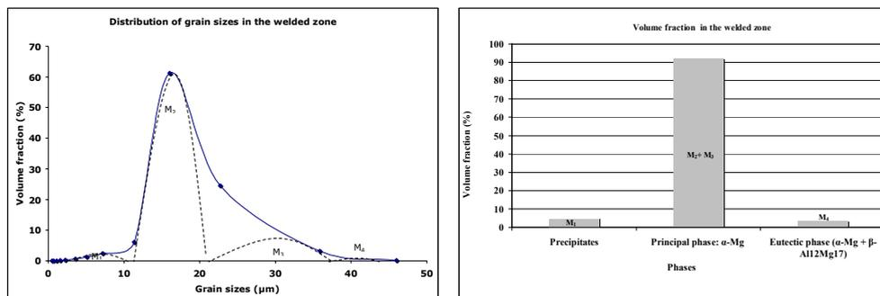
Fig. 6. a) Statistical distribution of the grain sizes of AZ91 alloys in welded zone, b) Volume fraction of the  $\alpha$ -Mg grains and of the  $\beta$ -Mg<sub>17</sub>Al<sub>12</sub> precipitates in the welded zone (Kouadri & Barrallier, 2010).
