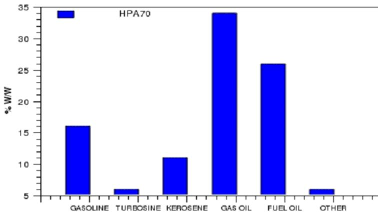
Fig. 14. Liquid products distribution obtained from the catalytic cracking of low-density polyethylene employing heteropolyacid-MCM-41 materials (Hernandez et al., 2010).
