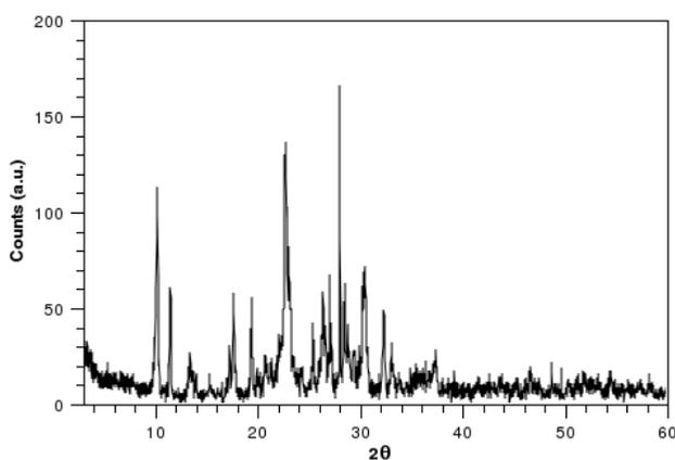
Fig. 2. X-Ray Diffraction pattern of natural clinoptilolite (Hernandez, 2011).
