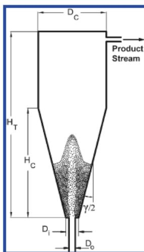
Fig. 11. Continuous spouted bed reactor (Elordi et al., 2011).
