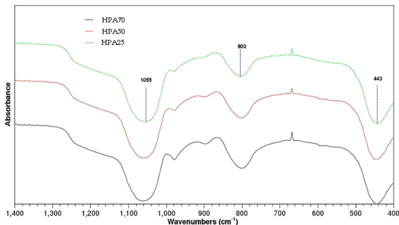
Fig. 8. FTIR spectra of heteropolyacid-MCM-41 materials. 25, 50 and 70 denote the w/w proportion of  $H_3PW_{12}O_{40}$  with respect to MCM-41.
