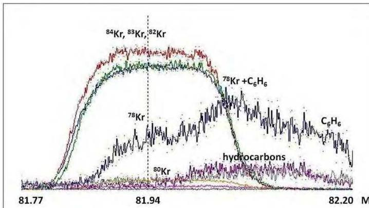
Fig. 4. Simultaneous detection of Kr isotopes 84, 83, 82, 80 and 78. Intentional fringe field distortion of the electrostatic zoom lens allows measurement of  $^{78}\text{Kr}$  without significant benzene contribution. Vertical scales (count rates) are different for different isotopes. Horizontal axis is mass for central (axial) isotope,  $^{82}\text{Kr}$  in this case. The assignment of ion collectors corresponds to step 4 of Table 1.
