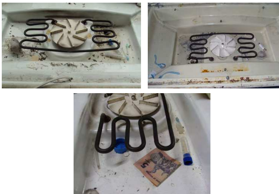
Fig. 11. Items of clinical and other materials trapped inside humidifier/heater chambers of three different incubators on active service.
