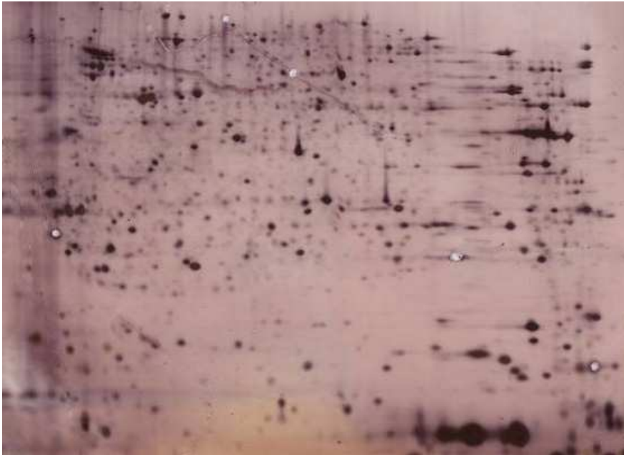
Fig. 2. Silver staining of acrylamide gel after SDS-electrophoresis Protein extract (600 \mu\text{g} ) from cerebellum was loaded in a first dimension IPG strip (pH3-11, NL, 24 cm; Running time: 15.5 hr, approx 47 kVh) and resolved in 12.5% acrylamide gel (Running time: 5.15 hr, 10 W per gel). Proteins were visualized by silver staining. These gels are called preparative gels, and they contain more protein content to allow for subsequent analyses including silver staining and MALDI-TOF. CyDye labelled proteins were run on analytical gels which are scanned by lasers and thus do not require a high quantity of proteins.
