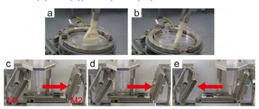
Fig. 3. Automated one-by-one sample preparation system. (a and b) Cell collection on the dish stage. (c-e) Process for elution of the protein complexes in the 'protein complexes elution device' (Fig. 1a). M1 and M2: magnets.
