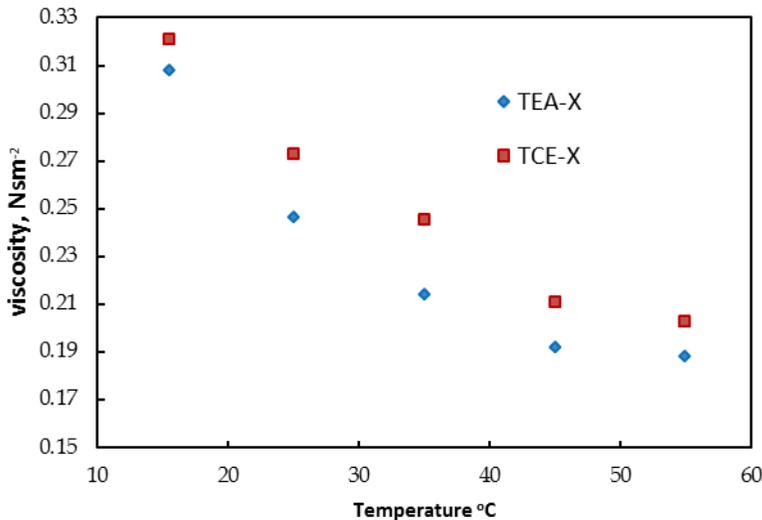
Fig. 3.7. Viscosity variation for doped sample II with temperature.
