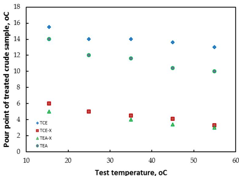
Fig. 3.8. Pour point depression test for sample II at varying test temperature.
