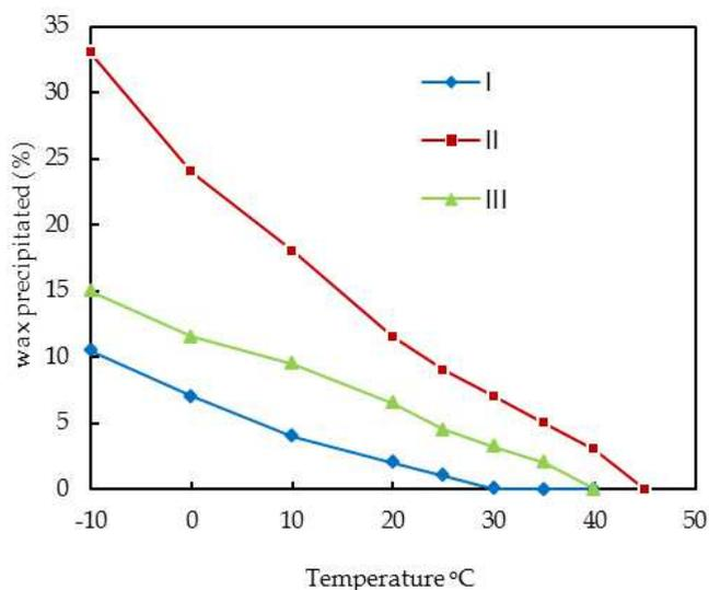
Fig. 3.4. Wax precipitation as a function of temperature.
