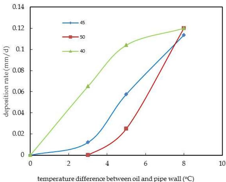
Fig. 3.6. Variation of deposition rate with temperature difference.
