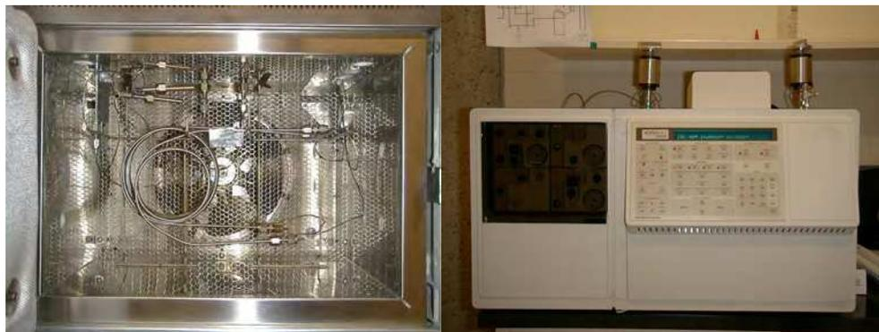
Fig. 5. Standard gas chromatograph and oven
