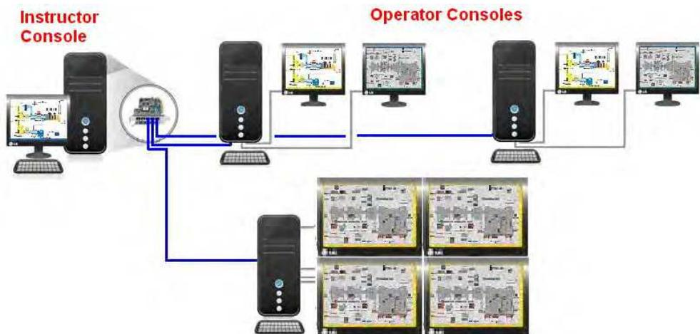
Fig. 11. Hardware architecture.
