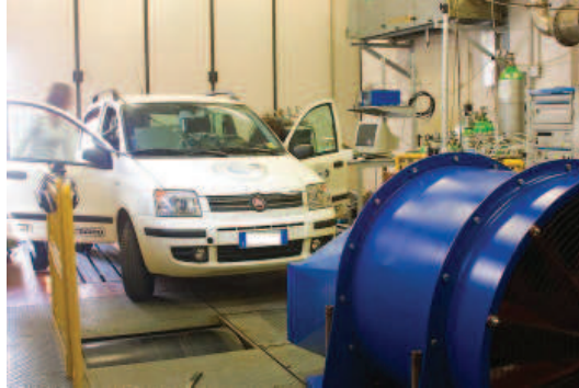
Fig. 16. Fiat Panda HCNG tested in the laboratory of Istituto Motori-CNR (Prati, Costagliola, Torbati, Unich, Mariani, Morrone & Gerini, 2011).
