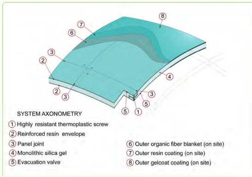
Fig. 12. F<sup>2</sup>TE<sup>3</sup> system axonometry
