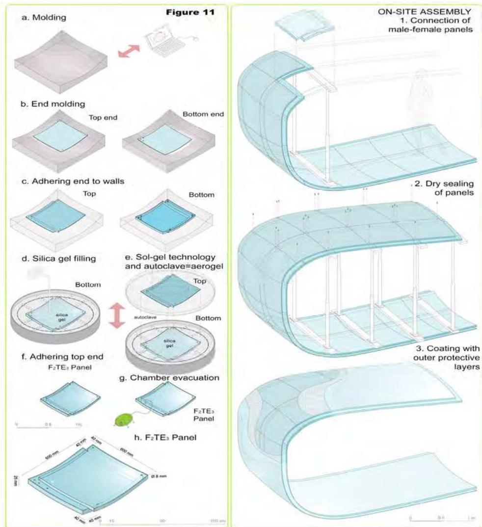
Fig. 13. Manufacturing and On-site assembly
