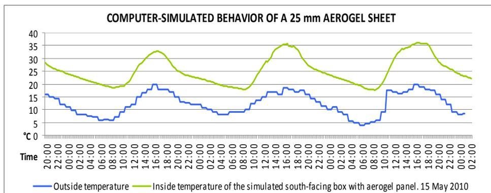
Fig. 4. Computer simulation for a 25mm thick sheet of silica aerogel with density 50-150kg/m<sup>3</sup> over 78 hours.
