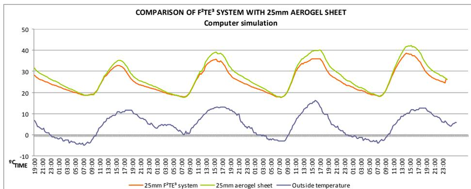
Fig. 14. Comparison of a computer simulation of a 25mm thick sheet of silica aerogel with a density of 50-150 kg/m<sup>3</sup> with the F<sup>2</sup>TE<sup>3</sup> system over 96 hours.
