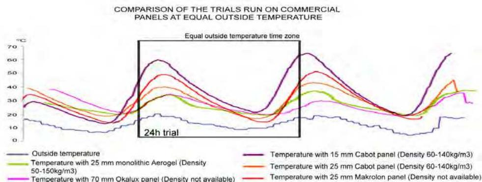
Fig. 10. Comparison of empirical data of commercial systems with computer simulation of 25 mm thick sheet of silica aerogel with density 50-150kg/m<sup>3</sup> over 78 hours (temperatures inside the test boxes)
