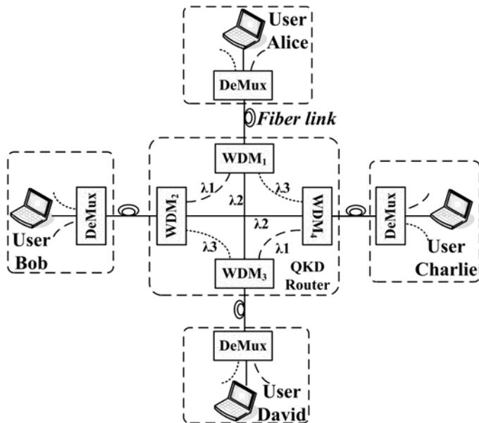
Fig. 12. Structure of four-user QKD router and the star network topology. DeMux: demultiplexer.
