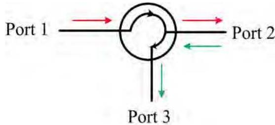
Fig. 8. The light path of optical circulator
