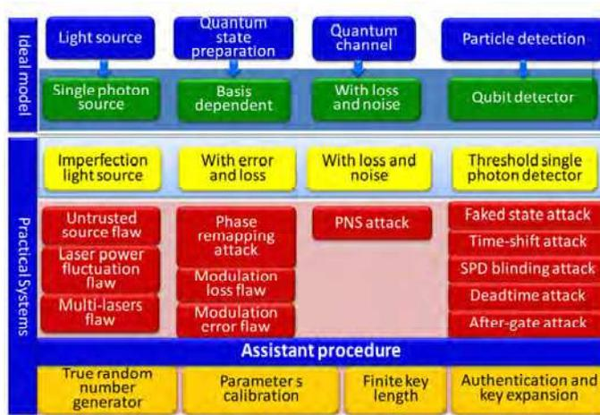
Fig. 3. The imperfections of practical QKD system and quantum hacking methods
