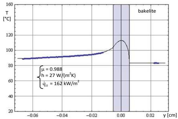
Fig. 9. Results for 0.57 m/s, 0.93 MPa
