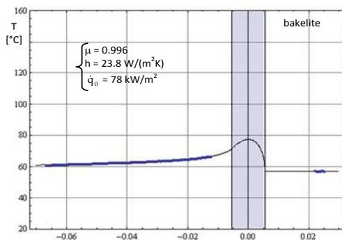
Fig. 11. Results for 0.28 m/s, 0.93 MPa
