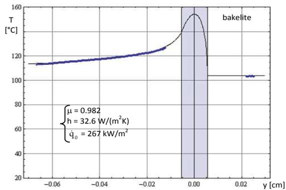
Fig. 10. Results for 0.57 m/s, 1.4 MPa
