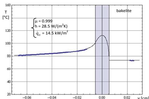
Fig. 12. Results for 0.28 m/s, 1.4 MPa
