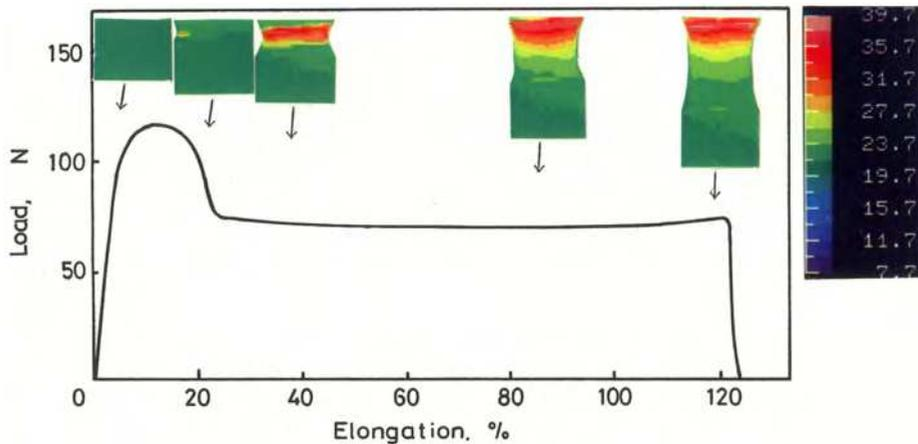
Fig. 26. Relationship of load-elongation, and some selected temperature distribution images of drawn PP film (Yamauchi, 2006).
