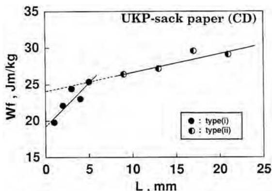
Fig. 22. Experimental determination of the specific essential work of fracture by extrapolation of the linear relation between work of fracture ( $w_f$ ) and ligament length ( $L$ ) for UKP-sack paper (CD) (Tanaka and Yamauchi, 2000).
