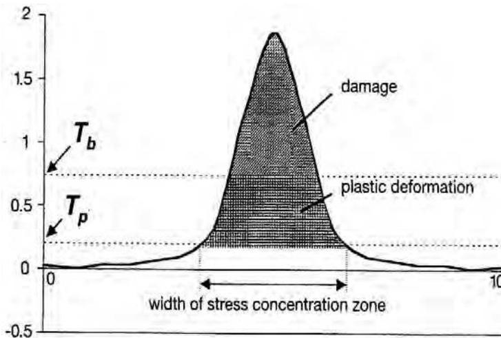
Fig. 25. Schematic image of threshold temperature. The curve shows the cross section of the 3-D image.  $T_p$ : threshold for plastic deformation and  $T_b$ : threshold for damage (fiber pull out or breakage) (Tanaka and Yamauchi, 2005).
