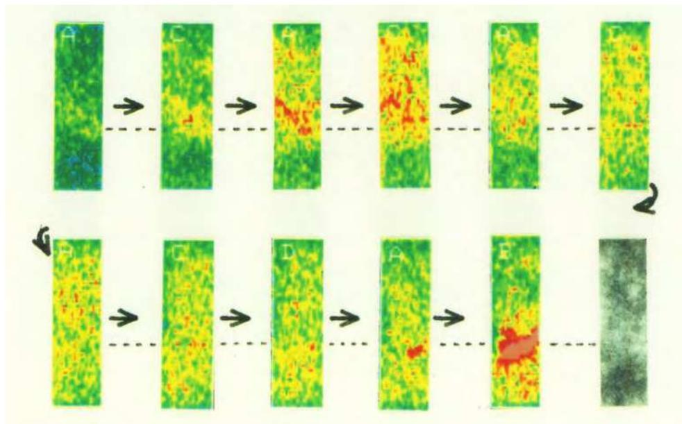
Fig. 10. Sequential subtracted temperature rise distribution images during straining and the soft X-ray mass distribution image of poorly—formed paper (Yamauchi and Murakami, 1994).
