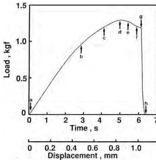
Fig. 17. Load-displacement curve for the UKP-sack paper (CD/L: 5mm) (Tanaka and Yamauchi, 2000).
