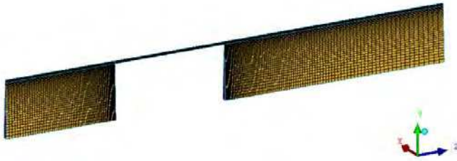
Fig. 11. CFD domain for the small sharp-edged cylindrical orifice case ( d=1 and l/d = 20 )
