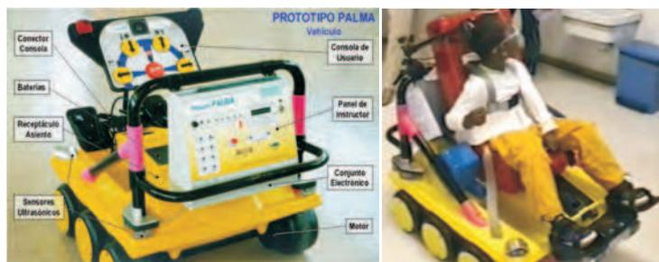
Fig. 1. Prototype PALMA project
